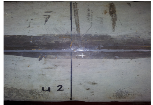
1mm cable embedded in 5x5mm groove
